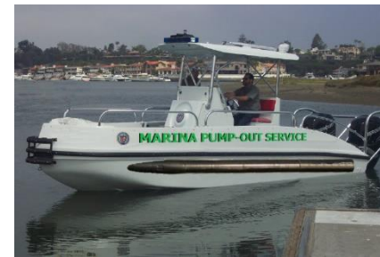
Zero discharge by waste pump-out
